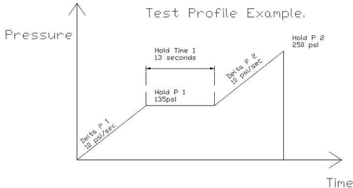
Note: it is important feature of pressure testing equipment to ensure the PRESSURE SET POINTS are being reached before beginning HOLD. If during a test the intended pressure was not being reached, before HOLD begins, a PET bottle is given more time to expand and as a result will burst at a lower pressure, additionally the PET bottle may be accepted as a 'pass' without ever having reached the intended pressure.
